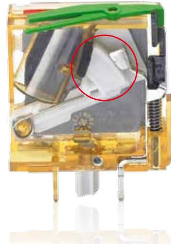
Exinction of the electric arc with the intervention of the patented device
