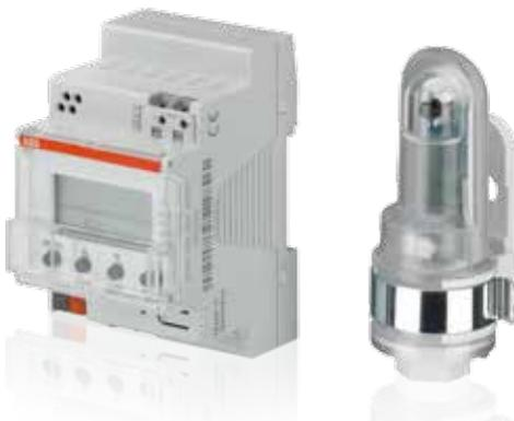
ABB's Outside Light Sensor Interface HS/S 4.2.1 measures the daylight brightness value and can be used as twilight sensor as well due to its very wide sensor range. It also offers a manual operation via a backlighted, text-based display, simplifying commissioning. One Outside Light Sensor LFO/A 1.1, which is required for measurement, is supplied with the device and up to 3 light sensors can be connected.
