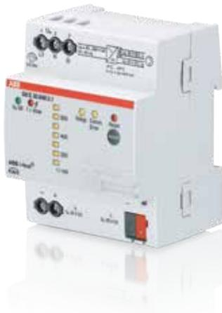
The new ABB i-bus KNX Power Supplies are equipped with an advanced LED display indicating the current bus load and offering a rapid diagnosis of the bus state. The state values are also provided via communication objects to the KNX system. Additionally, the ABB i-bus Tool enables a detailed analysis of actual values. The connection to the KNX is established via a bus connection terminal. All other connections are made via terminals equipped with a universal head screw.
