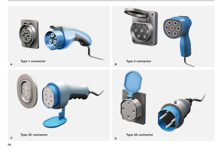
**Type 3C connector** (see figure 04c) as per IEC 62196-2. In use as socket-outlet fr charging stations mainly in France. Its characteristics are similar to those of the type 2 socket, but it is mechanically incompatible with this.
