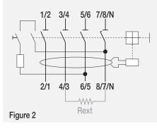
To permit operation of the test button also for three-phase networks without neutral with line voltage of 400 V between the three phases, the phases must be connected normally (inputs to terminals 1/2, 3/4, 5/6 and outputs to terminals 2/1, 4/3, 6/5), and insert a resistor between terminals 4/3 and 8/7/N of the RCD, as shown in figure 2, the value of which is given in table 1 (based on the RCD sensitivity).
