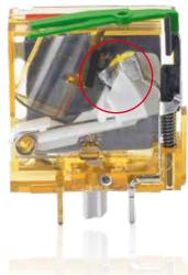
At the end of life, opening of the thermal disconnector and ignition of an electric arc in direct current
