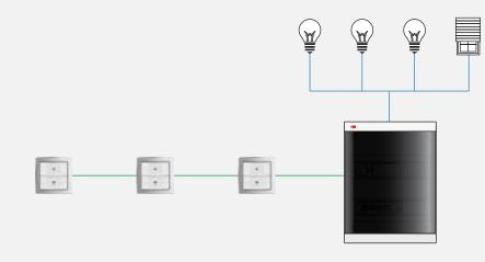
03 Controlling lighting from multiple points via decentralised KNX installation.
