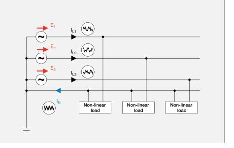
$$I_N = 3 \times \sqrt{I_3^2 + I_9^2 + I_{15}^2 + \dots}$$
