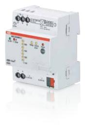
The new ABB i-bus KNX Power Supplies are equipped with an advanced LED display indicating the current bus load and offering a rapid diagnosis of the bus state. The state values are also provided via communication objects to the KNX system. Additionally, the ABB i-bus Tool enables a detailed analysis of actual values. The connection to the KNX is established via a bus connection terminal. All other connections are made via terminals equipped with a universal head screw. Two devices are available:
