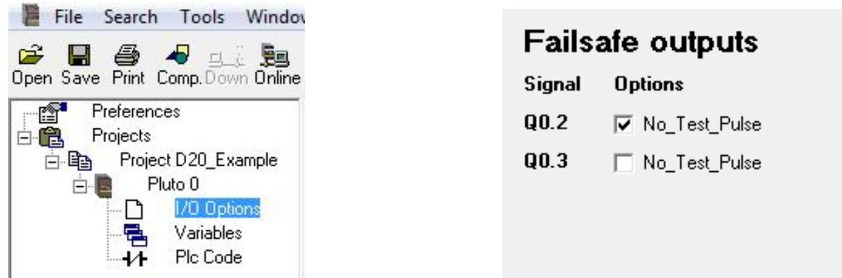
The screenshot shows the Pluto Manager interface. On the left, a tree view shows the project structure: Preferences, Projects, Project D20\_Example, Pluto 0, I/O Options (highlighted), Variables, and Plc Code. On the right, a panel titled 'Failsafe outputs' contains a table with two rows: Q0.2 and Q0.3. The 'Options' column for Q0.2 has a checked checkbox for 'No\_Test\_Pulse', while for Q0.3 it is unchecked.
