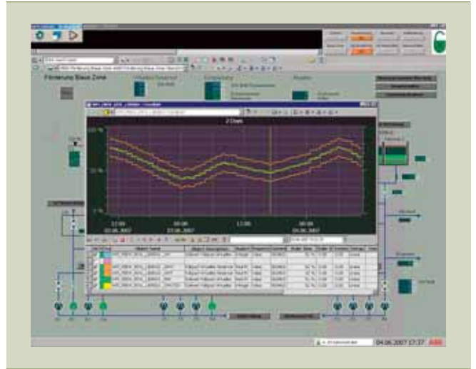
3 Filling the virtual reservoir: the actual level (green) follows the optimal set-point (yellow) and stays within the tolerance limits (orange)
