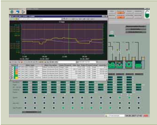
2 Status of water wells. In this example, the flows from the different wells (blue, green and yellow) are equal
