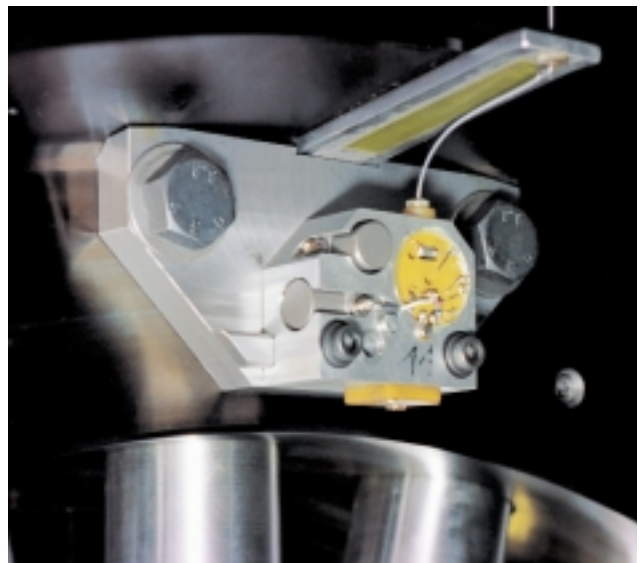
9 Transmitter casing with integrated accelerometers
