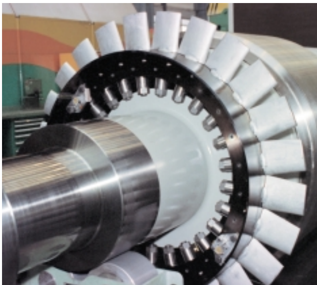
8 500-MVA turbogenerator equipped with two accelerometers at the hub of the axial fan
