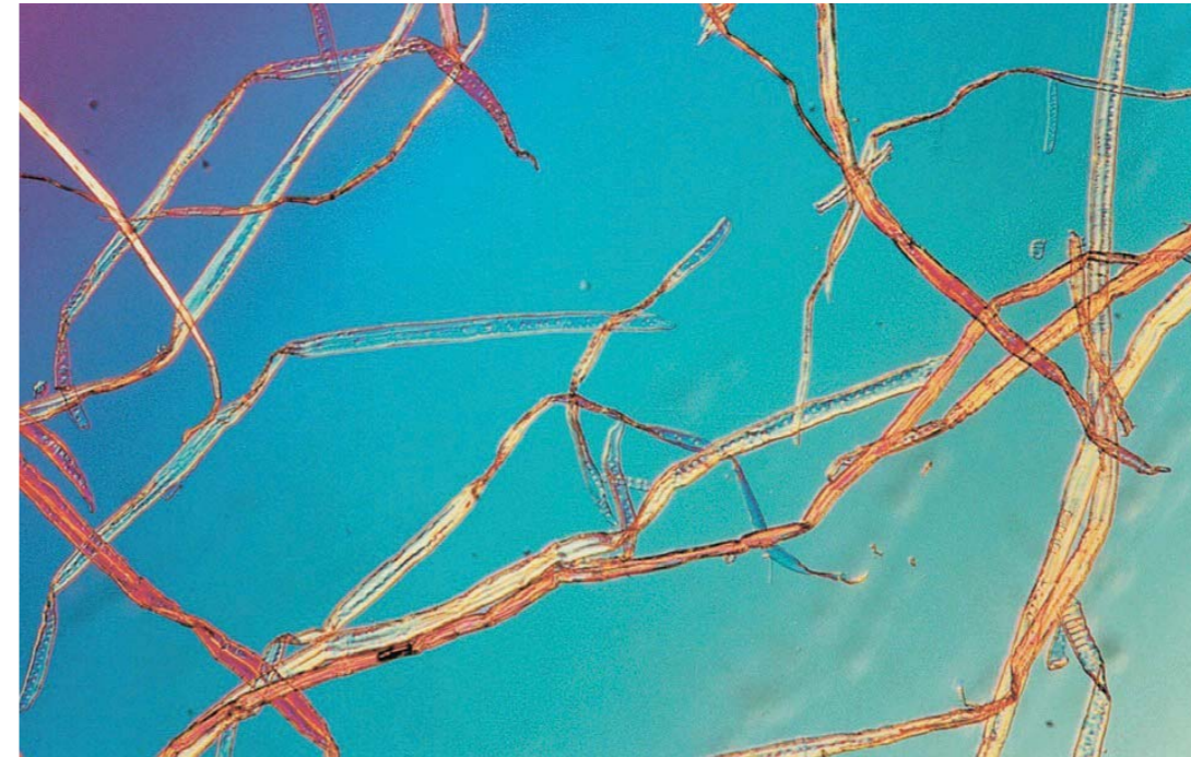
Figure 2: Bleached softwood fibres, 50 times magnification
