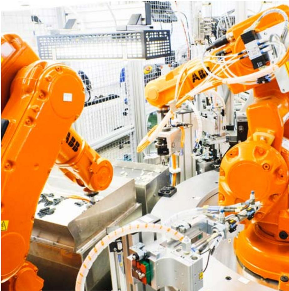
The robots only require supervision by one operator, and they process about 8,500 pieces per shift.
