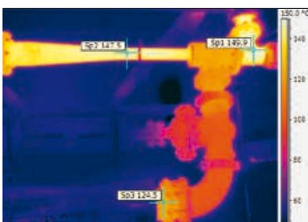
Cooler flash steam enters at 124.6 °C. High pressure motive steam enters from the right at 149.9 °C, giving a 147.5 °C mix, which is close to the motive steam temperature, hence very little flash steam is recycled.
