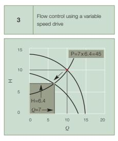
of the pump due to different speeds and geometric similarity. To be more specific, the power required to run a pump is proportional to the cube of the speed. This means that if 100% flow requires full power, 75% requires (0.75)<sup>3</sup> = 42% of full power and 50% flow requires 12.5% of the power.
