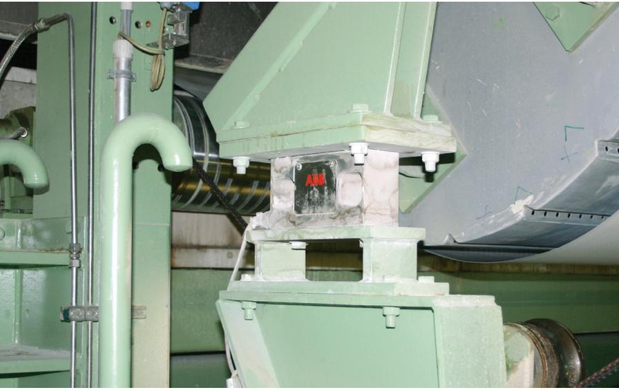
The paper machines and the three coating machines are running with PillowBlock load cells providing an accurate web tension measurement.
