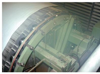
01-02 ABB Pressductor PillowBlock load cells mounted at the air turn application in the coating machine.
