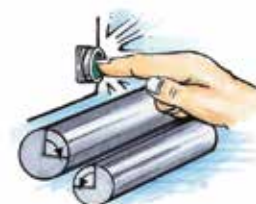
Shaft only turns a small amount each time the PB is pressed.
