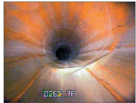
4 B-scan display of weld area and video record of internal condition of pipe
