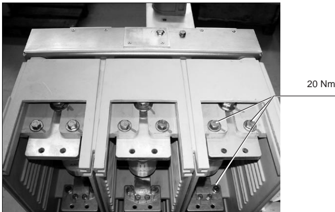
Figure 12: Terminals Torque Requirements
