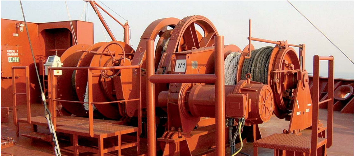
The Pusnes frequency controlled winch™ includes an ABB industrial drive with winch control program.
