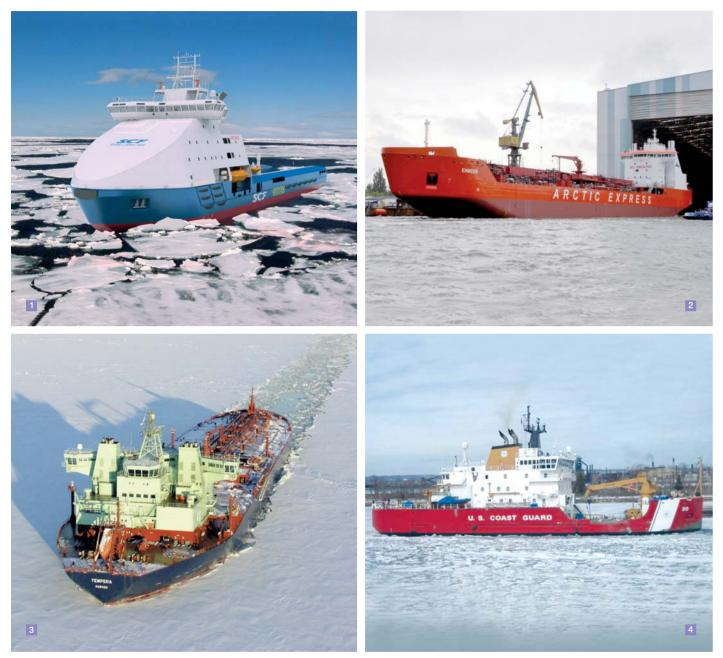
1. Newbuilding – icebreaking PSV. 2 x 6.5 MW Azipod propulsion. Owned by Sovcomflot, and built by Arctech Helsinki Shipyard.
