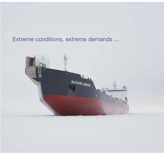
Sovcomflot's Arctic shuttle tanker MT Vasily Dinkov and her sister vessels are equipped with 2 x 10 MW Azipod VI propulsion systems.
