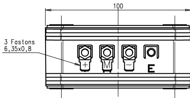
The internal screen (E) is connected to -V<sub>A</sub>
