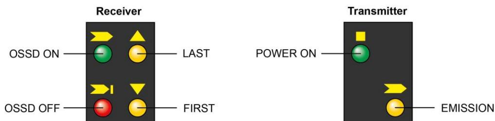
The meaning of the LEDs on the receiver (RX) depends on the AOPD operating mode.
