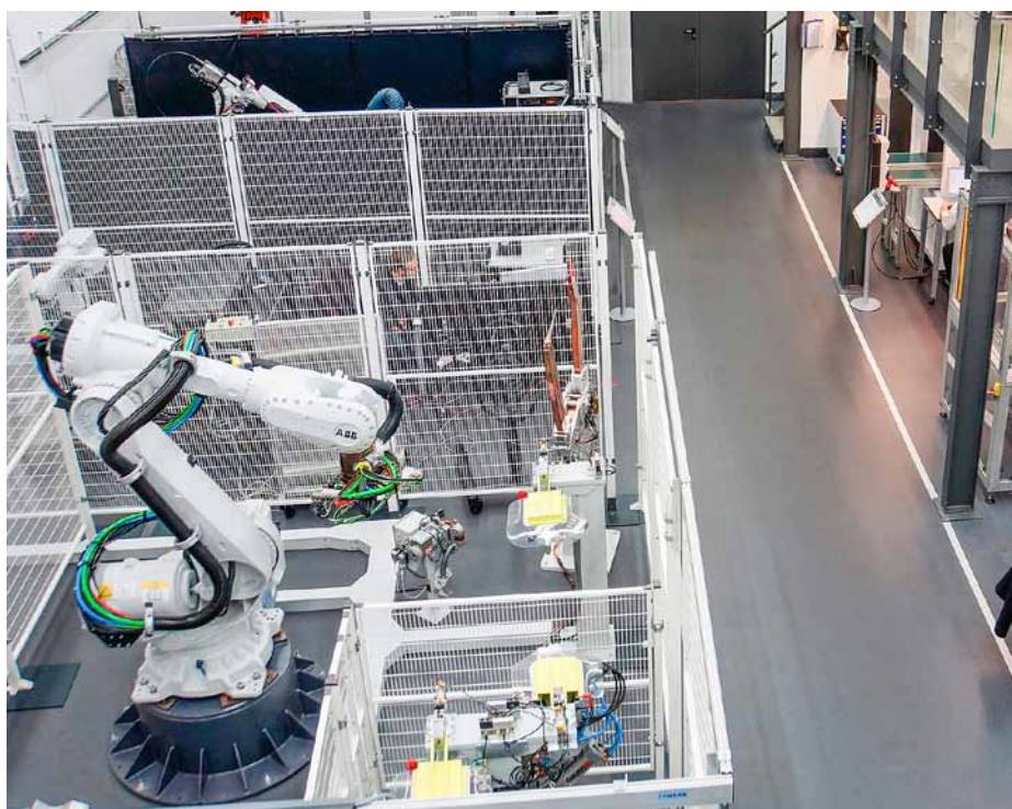
Robots operating in a sand core cell on a cylinder heads manufacturing line in China.
