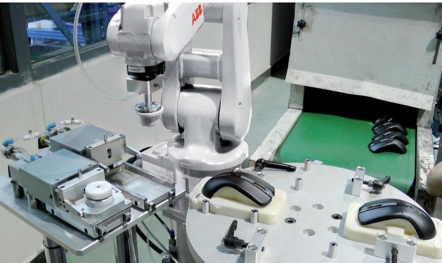
On the production line of the Rapoo computer-peripheral plant in Shenzhen, China, 80 of ABB's IRB 120 robots are hard at work. The robots – ABB's smallest – are responsible for assembling wireless mice, keyboards and their sub-components. They've also enabled Rapoo to overcome two major production problems – a shortage of skilled labor and a need for design flexibility.
