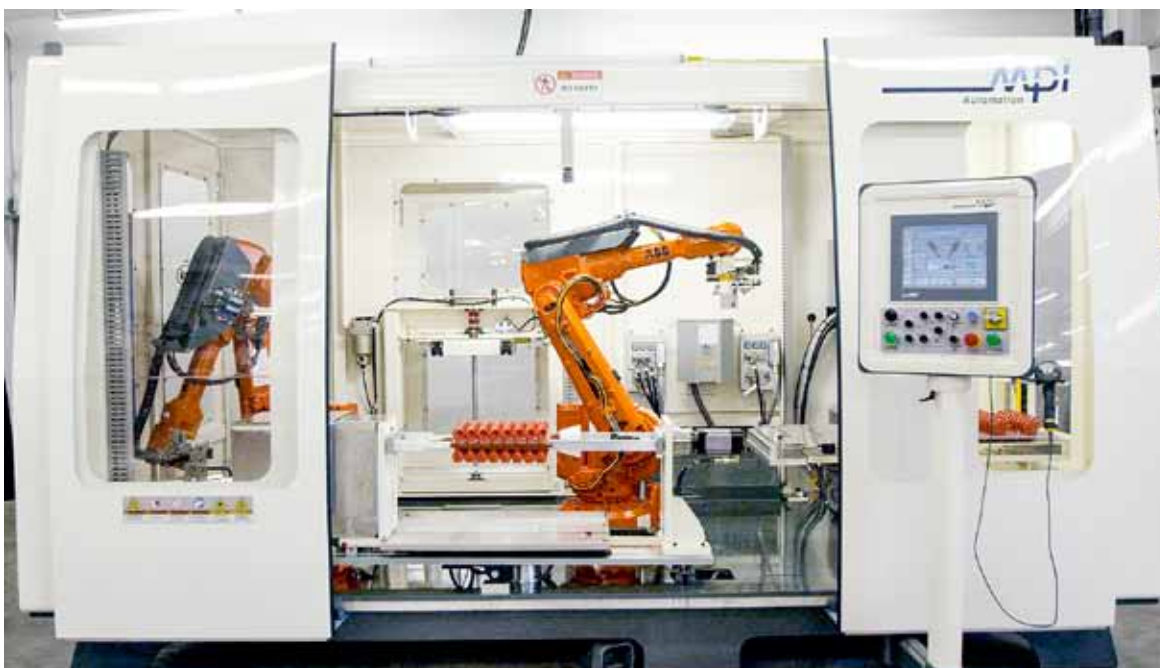
MPI's new model 20-14 automated pattern assembly system uses two IRB 2600 6-axis robots.
