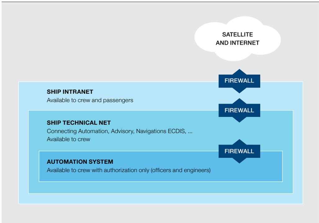
architecture and how the network is connected with other systems on the ship and on land. The key word here is defense-in-depth, with security zones in place. Defense-in-depth refers to multiple, independent and redundant layers to compensate for potential human and mechanical failures so that no single layer, no matter how robust, is exclusively relied upon.
