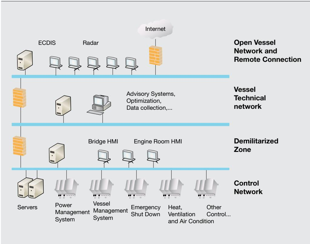
Technical Net (see Figure 1). It could be connected through a firewall to an open ship network, which is then connected to the world through a satellite link.
