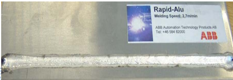
Rapid Aluminium Welding
