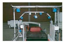
Last autumn, ABB Airport Technology, in close cooperation with ABB Corporate Research, installed a pilot automated baggage loading system in Zurich airport. The very successful performance of the installation has shown that the combination of known technologies (IT, instrumentation, robotics, mechatronics) with application know-how has given ABB the lead in this new, fast-growing market. No comparable solution is offered by any other company.
