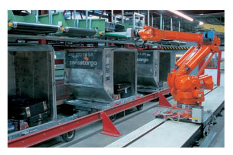
Two basic interchangeable tools are enough to solve most baggage handling problems.
