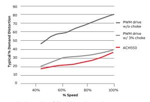
55% less harmonics at full load, better than 64% less harmonics at partial loads. (HVAC drives spend most of their operating hours at partial load.
