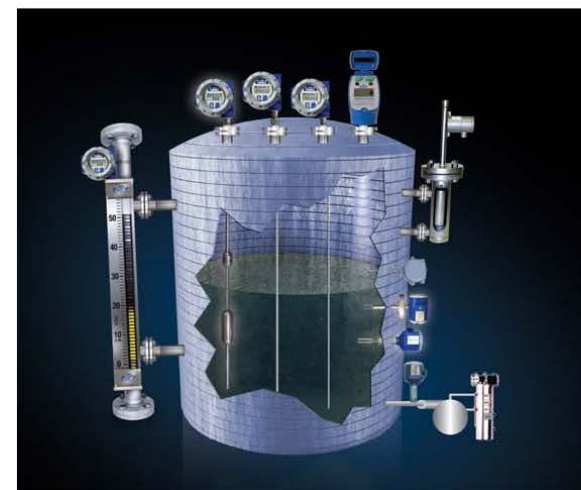
Figure 1: Level Measurement determines the position of the level relative to the top or bottom of the process fluid storage vessel. A variety of technologies can be used, determined by the characteristics of the fluid and its process conditions.
