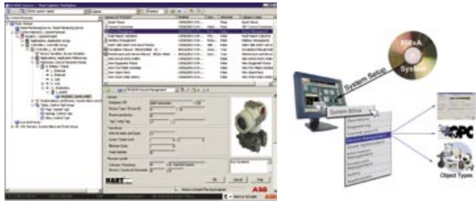
Figure 7. 800xA Fieldbus Management Tool supporting HART device parameters and connection via HART OPC
