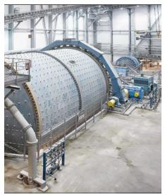
An example of an industry-standard comminution circuit providing high throughputs can be seen in  $\rightarrow$  3. This circuit, however, has a high specific energy consumption per ton of ore processed, driven primarily by the low efficiency of the ball mills and the need to use steel media for grinding.
