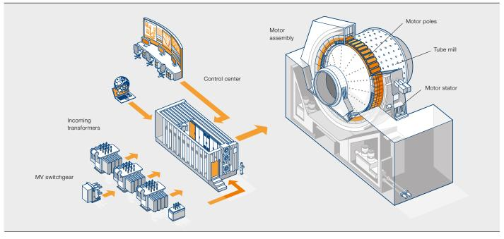
The advantages of a GMD application in the minerals grinding process have been well established over the past 40 years, with the benefits increasing exponentially as the mills get bigger.
