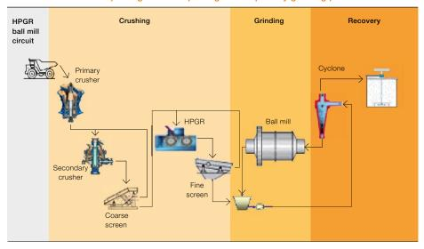
HPGRs are poised to play an important role in the comminution circuits to help reduce energy costs, water requirements and footprint compared with the traditional SABC circuits. While being a standard solution in mineral processing, HPGR technology continues to undergo constant development. ABB is at the forefront of this development with many new features being added to further optimize drive system performance.
