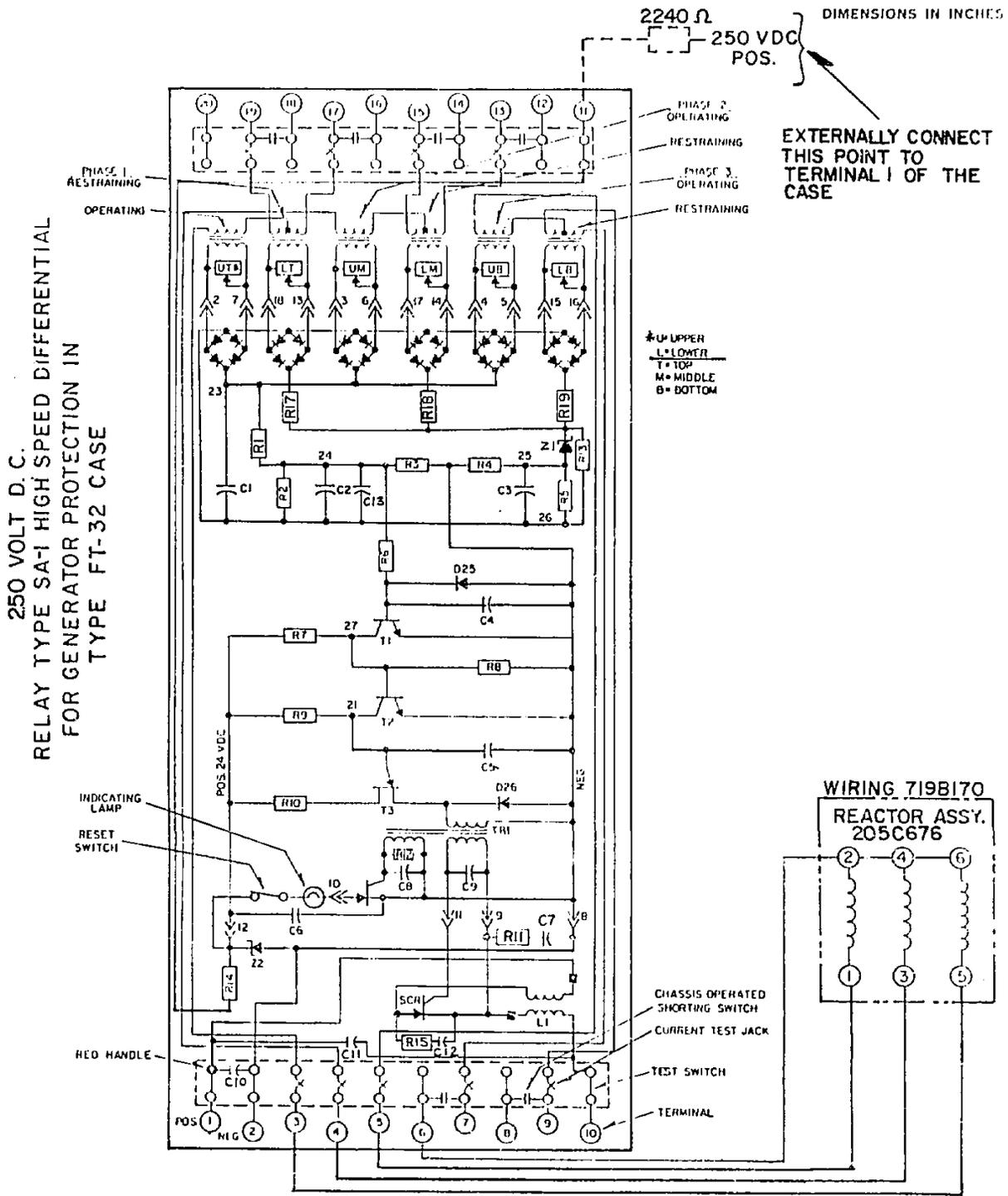
Figure 4. Internal Schematic of Type SA-1 Relay 250 Vdc
