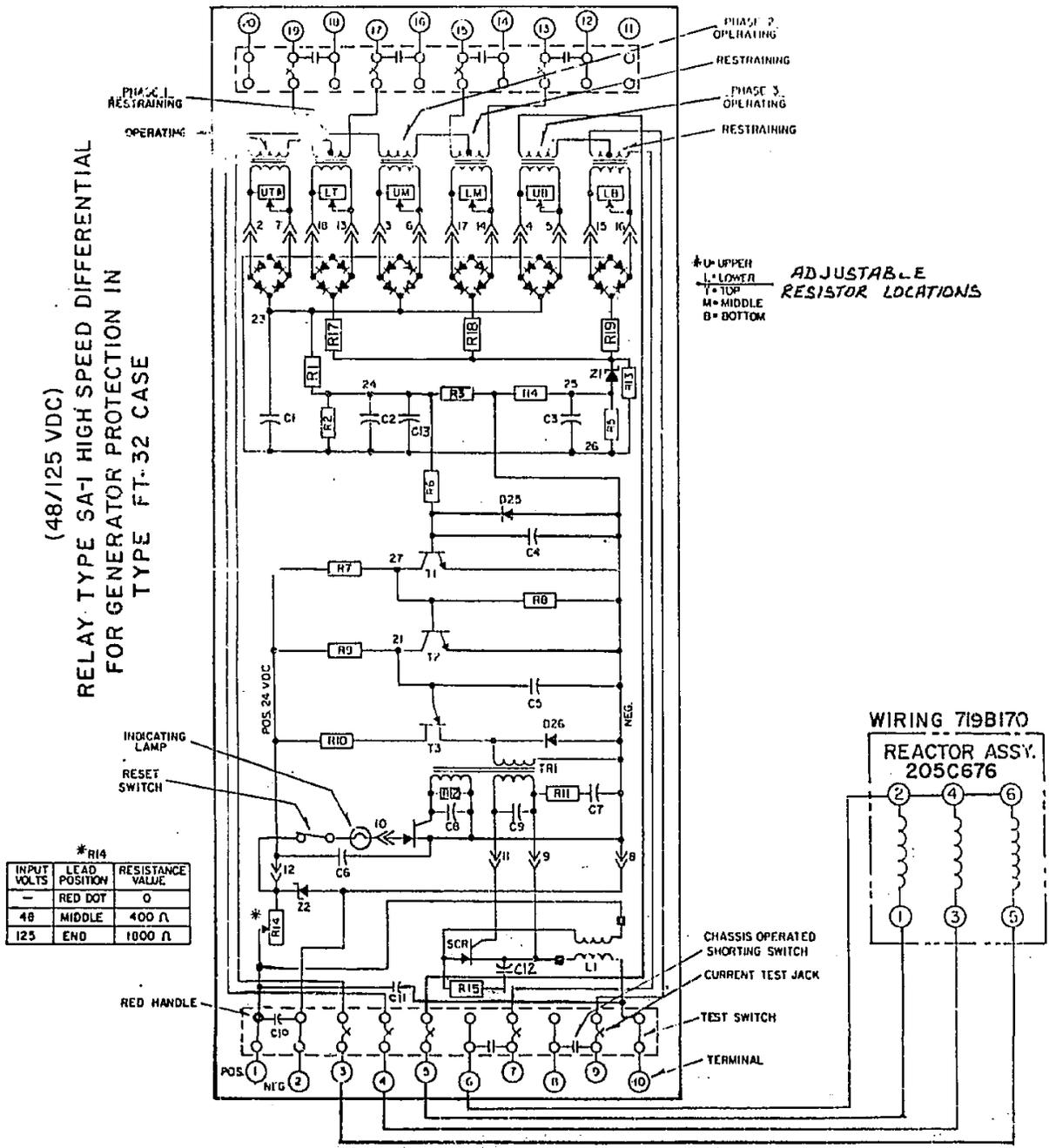
Figure 3. Internal Schematic of Type SA-1 Relay 48/125 Vdc
