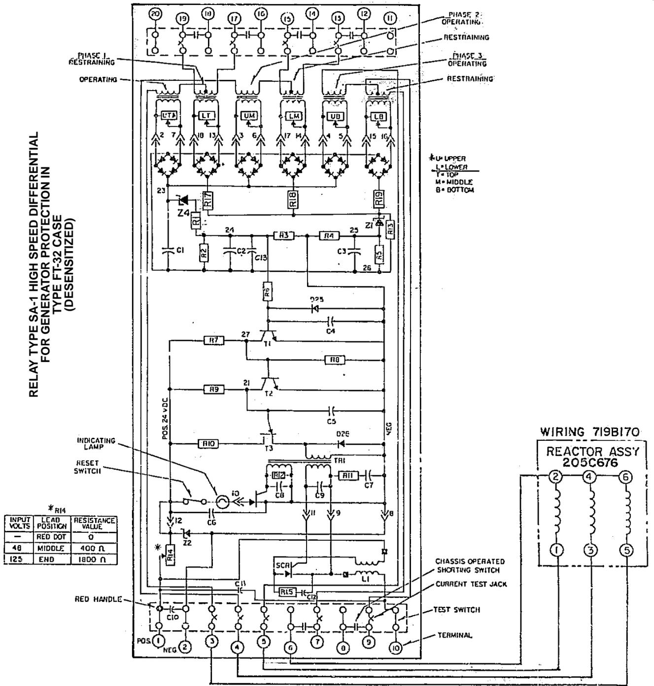
Figure 5. Internal Schematic of Desensitized SA-1 Relay
