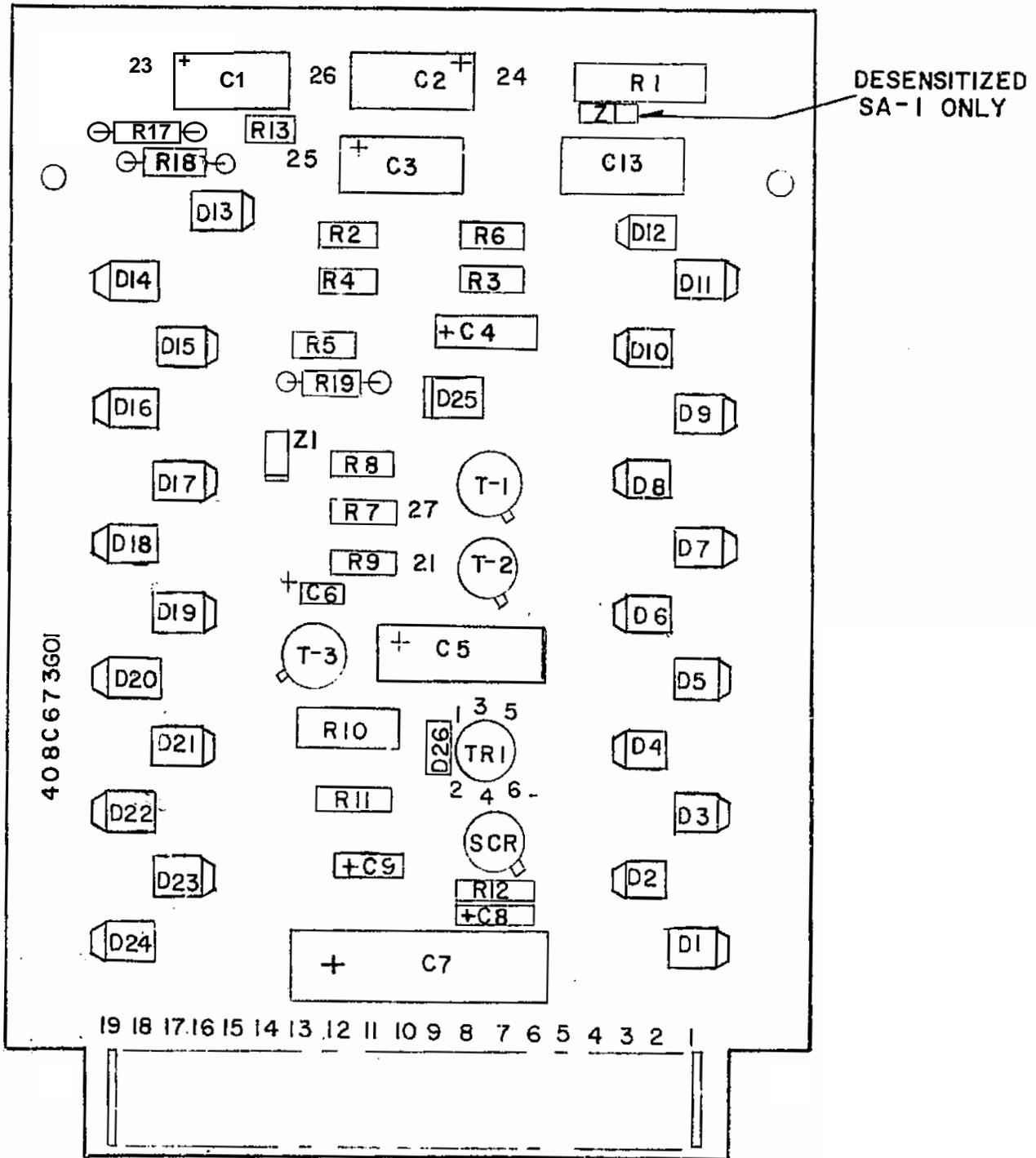
Figure 6. Component Location for 48/125 Vdc
