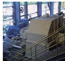
View of the cane mill (862 kW) and ACS1000 controlling the cane mill at Santa Matilde mill of Compañía Azucarera Hondureña S.A.
