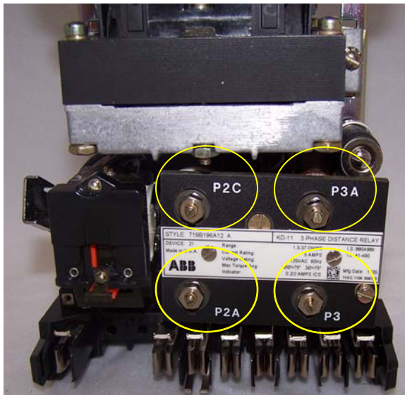
P2C, P3A, P2A and, P3 added for ease of calibration and maintenance
