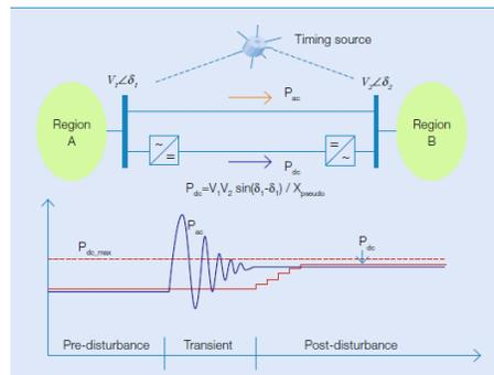
**Figure 8:** AC line emulation in post-disturbance situation
