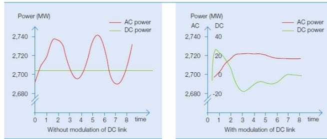
**Figure 7:** WAMS enabled control for power oscillation damping
