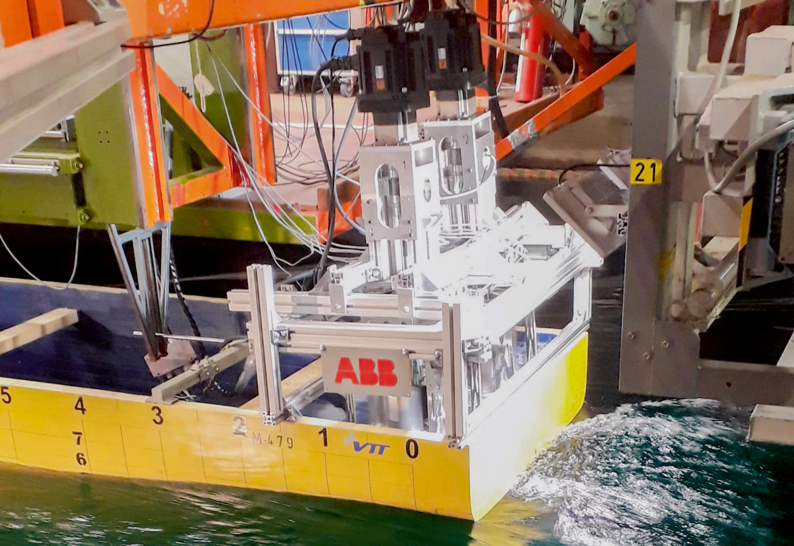
— Figure 1: Scale-model testing by VTT at the Otaniemi (Finland) towing tank
