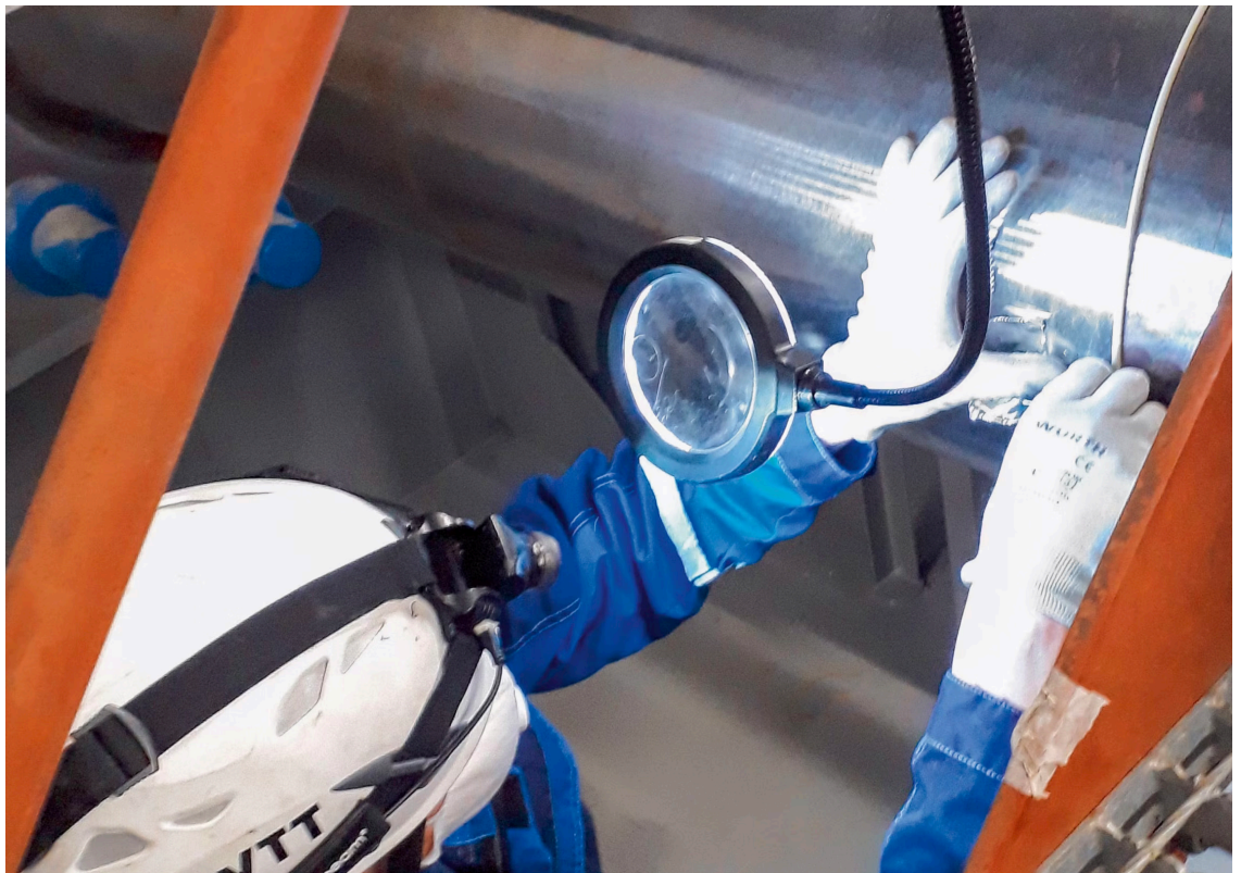
— Figure 4: VTT possesses all the skills in-house for the complete engineering of test environments. Here, a VTT engineer is installing instrumentation to a ship propeller shaft in preparation for sea trials
