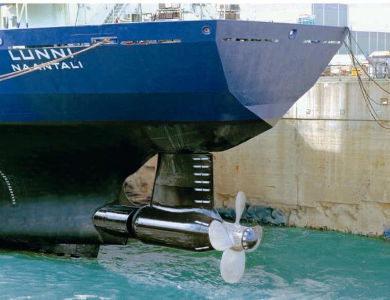
— Figure 3: MT Lunni after conversion to 11,4MW Azipod propulsion (left) and a view of the ship in a rubble field in astern mode
