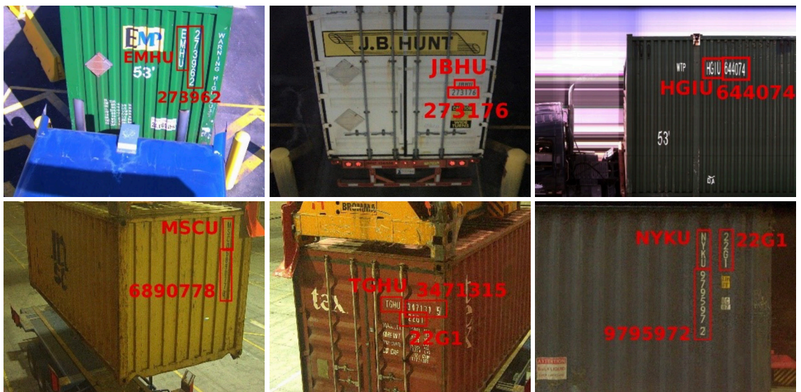
Figure 4: Example outputs of the container ID OCR system for ISO/ Domestic ID containers
