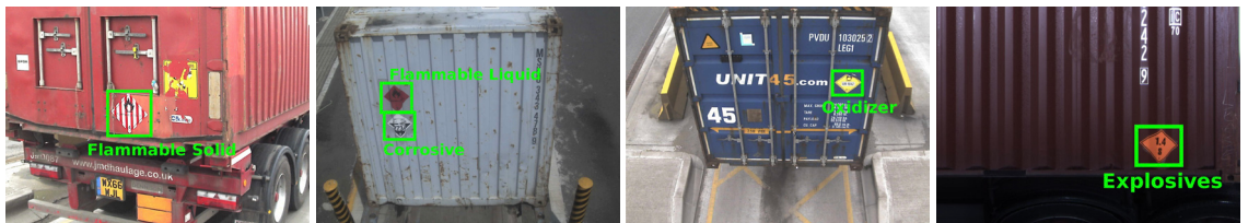
Figure 9: Example outputs of the hazmat placard detection and recognition system
