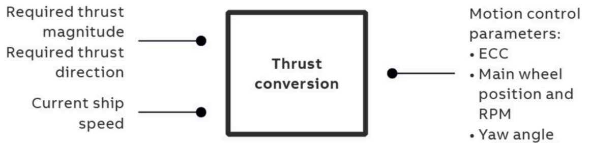
Figure 1: Thrust conversion: required thrust magnitude and direction is converted to motion control parameters
