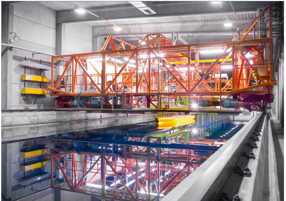
— Figure 3: The VTT towing tank is large enough for comprehensive scale-model testing
