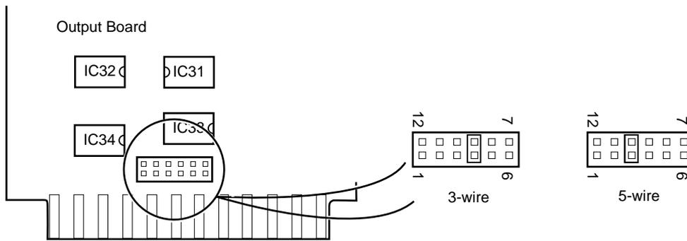
**Fig. 4.2 Serial Connections**
