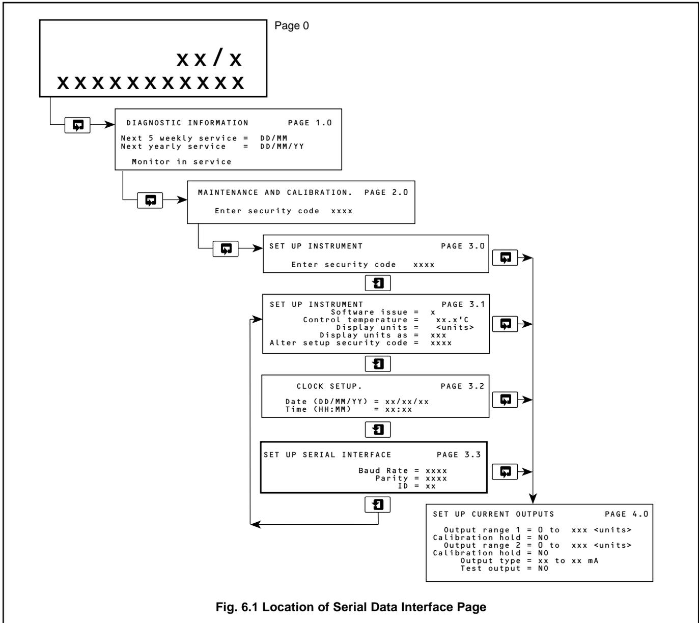
Fig. 6.1 Location of Serial Data Interface Page
