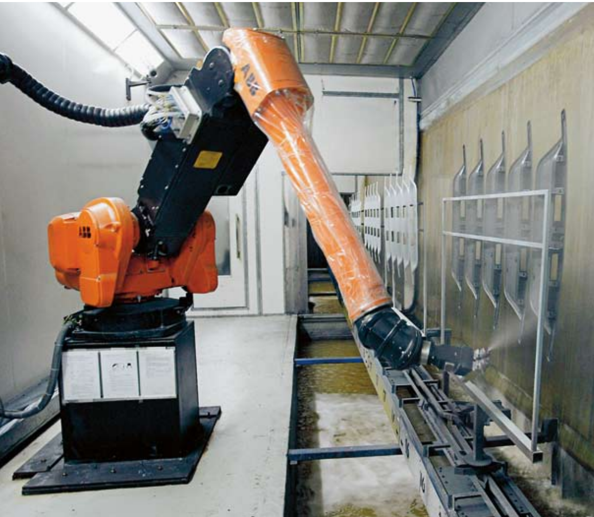
An IRB 5400 robot spraypaints the backs of rear parcel shelf brake light housings at D&M.
