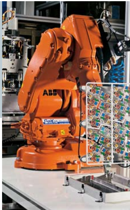
A 6-axis IRB 140 robot mans the injection moulding.
