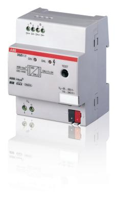
The DALI Gateway 1-fold DG/S 1.1 controls an unlimited number of lighting groups that are only limited by the max. number of KNX associations. 64 DALI devices can be individually switched on/off, dimmed and controlled via a brightness value using KNX. Further individual functions are possible with an address-based control.
