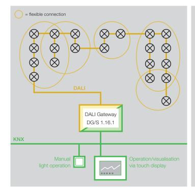
The new DALI Gateway DG/S 1.16.1 controls 16 flexible lighting groups with up to 64 DALI devices – also ideal for simultaneous switching and dimming of larger lighting groups.
