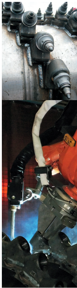
The operation to place and weld the teeth takes 10 hours, manually the process would take up to 100 hours.
