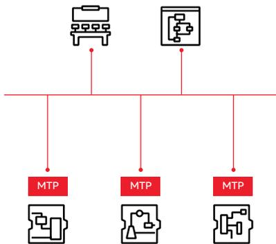
**Step 3:** A modular architecture still uses a central controller, but it needn't be anywhere near as powerful since control functions are distributed to smaller, less expensive controllers governing each module.
