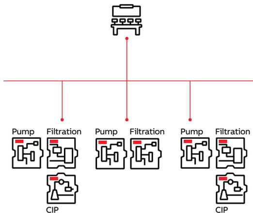
**Step 4:** Modules are thus equipped with their own intelligence to allow them to carry out tasks with less reliance on the master controller. Parts of a process can now be inserted, removed or adapted without affecting others around it.
