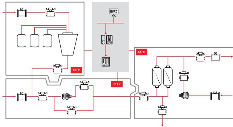
**Step 2:** Individual modules are pre-automated and then added together, like Lego blocks, to create a process line function. Each block acts as a plant within a plant, equipped with its own control functions and intelligence.
