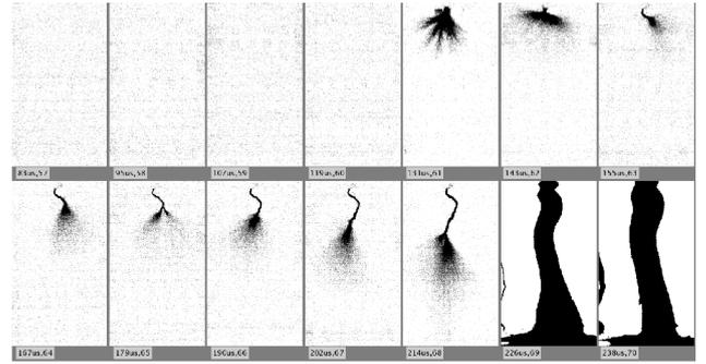
Figure 2. Leader propagation path for 3 m gap distance for 0.5 m diameter sphere– plane arrangement under positive switching impulses. The picture was taken with 84000 FPS and 11.9  $\mu$ s per frame.
