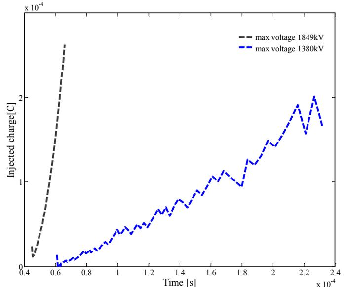
Figure 4. Injected charge to the leader channel.
