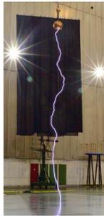
Figure 1. Breakdown photograph for sphere 0.5 m – plane arrangement under positive switching impulses
