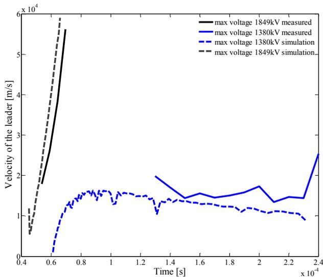
Figure 3. Leader propagation velocity for overvoltage and non-overvoltage condition.
