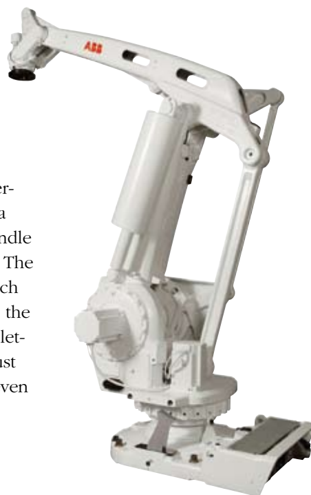
IRB 660, blending speed, reach and payload for the most demanding palletizing applications
