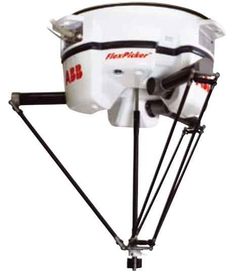
IRB 360 , Improved cycle time - up to 20%, Payload 3 kg - up 50%, Reduced footprint - 35% smaller
