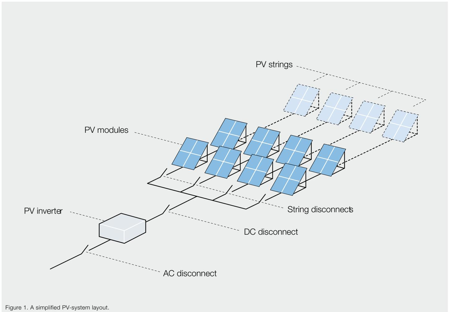
Figure 1. A simplified PV-system layout.
