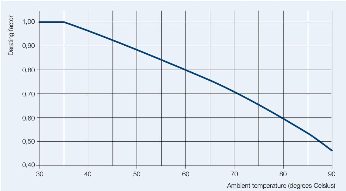
Figure 3. Estimated derating Factor, Function of Temperature (°C).
