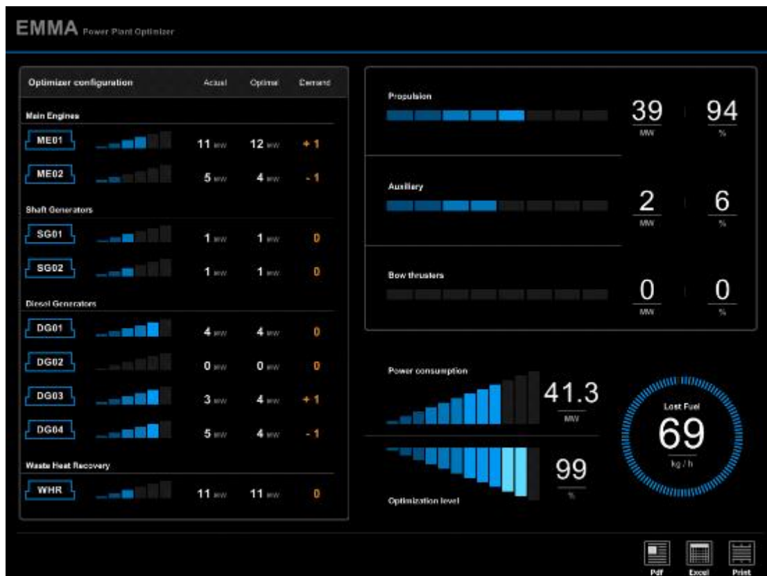
Figure 8: EMMA's power plant optimization user interface
