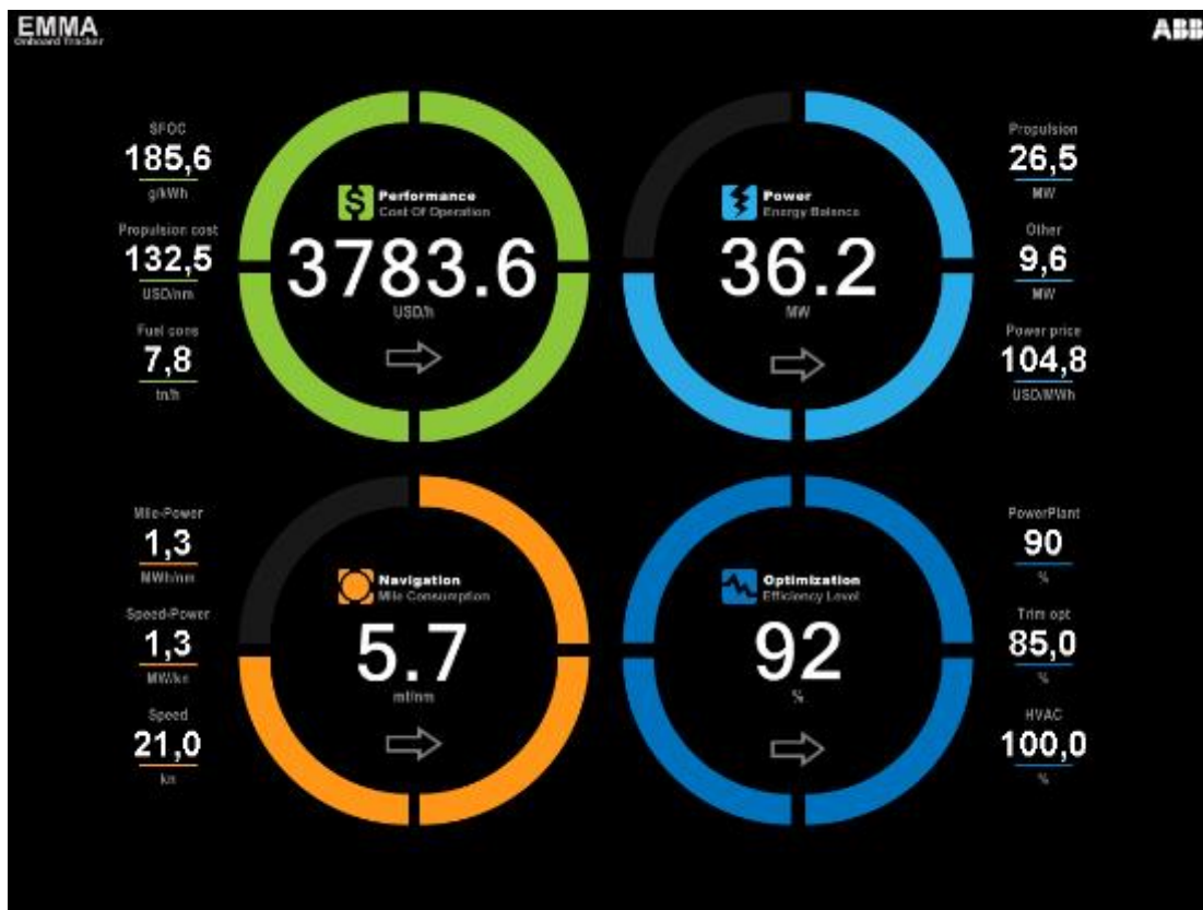
Figure 3: EMMA uses adaptive targets to provide the operating crew with realistic goals
