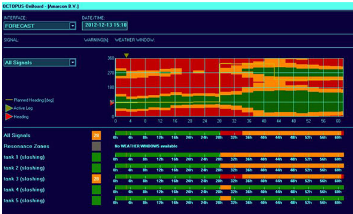
Figure 7: OCTOPUS forecasts the risks for sloshing for each individual LNG tank onboard LNG vessels
