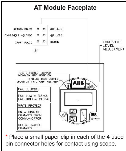
**Channel A:** Refer to the drawing at left for probe connections.\*
