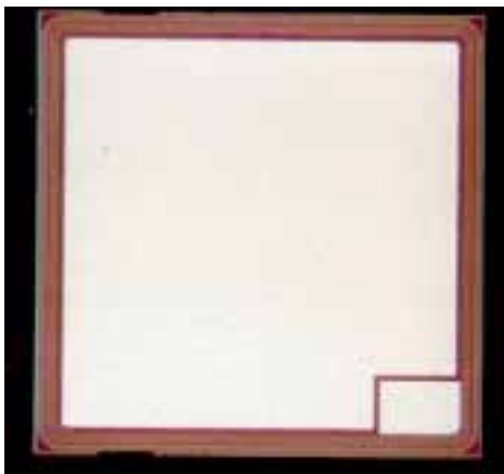
Fig. 6 IGBT Die showing corner gate pad and large emitter bonding area
