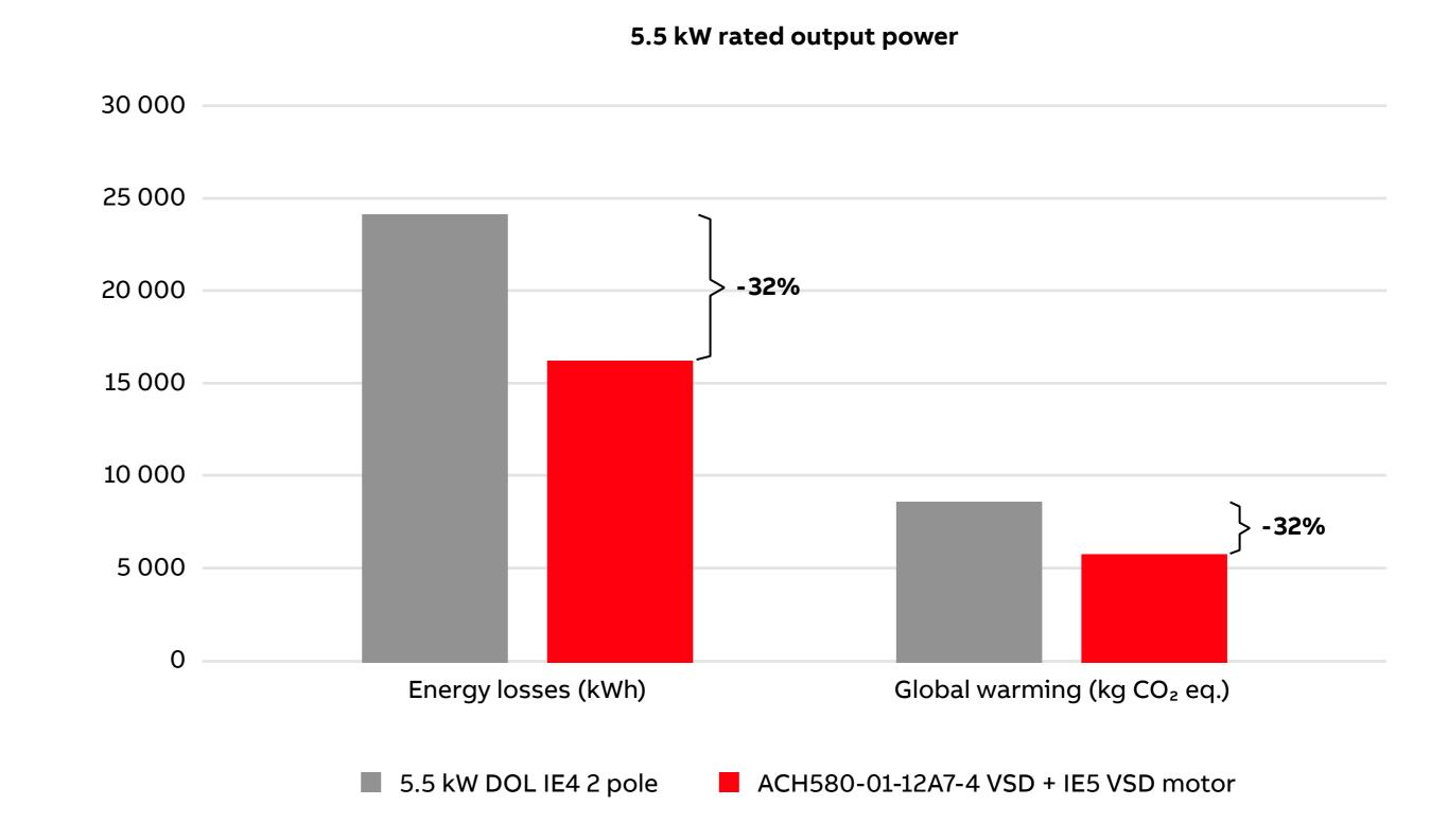
Use stage energy losses and contribution to global warming of ACH580-01-12A7-4 VSD + IE5 VSD motor system and an equivalent DOL motor.
