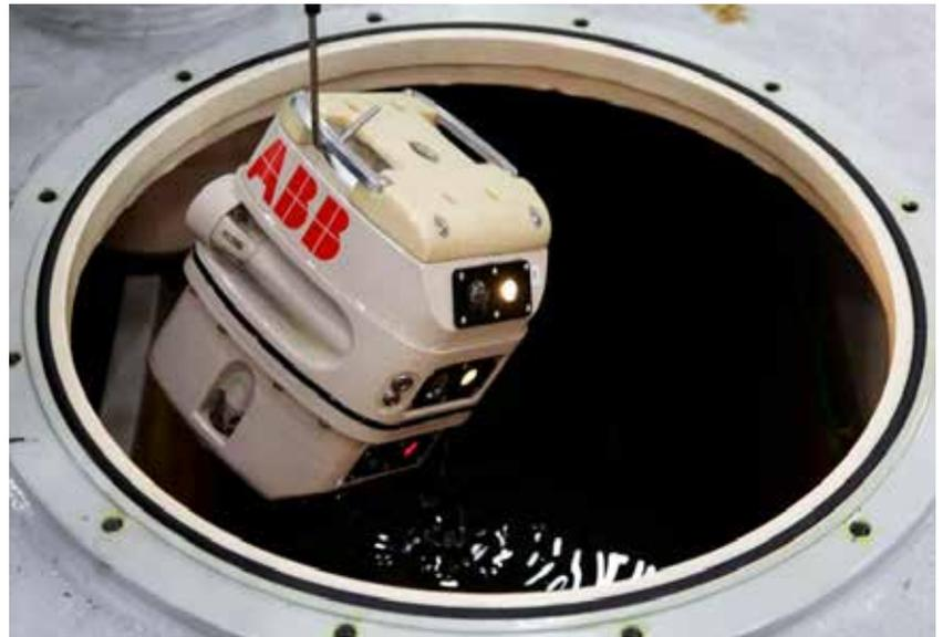
TXplore™ inspection robot being inserted into a power transformer
