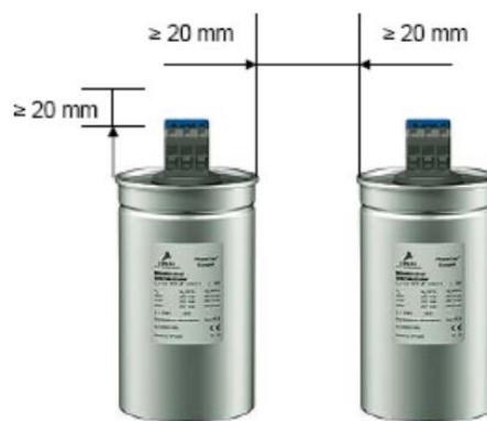
Figure 3: Minimum space over and between the capacitors.
