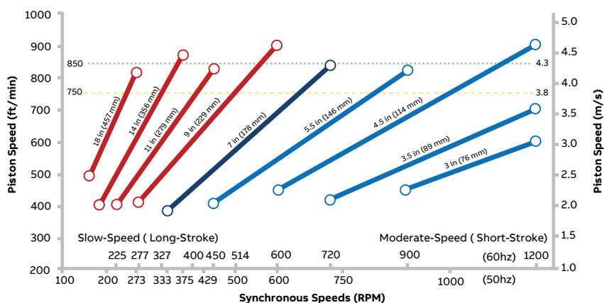
02 Ariel moderate-speed process compressors operate in comparable piston speed ranges to long-stroke, slow-speed compressors.
