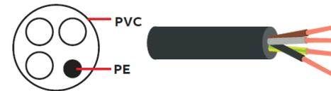
A 4-conductor system (3-ph. conductors and PE in a PVC conduit) is allowed for input cabling with phase conductor cross-section less than 10 mm<sup>2</sup> or motors < 30 kW. Not allowed in the USA.
