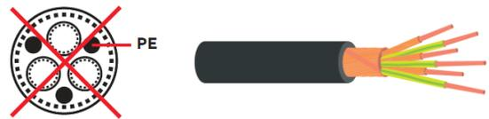
Symmetrical shielded cable with individual shields for each phase conductor is not allowed on any cable size for input or motor cabling.
