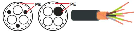
Symmetrical shielded cable with 3-ph. conductors, 1 or 3 symmetrically constructed PE conductors and shield. PE conductor must meet IEC 61439-1).
