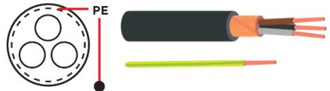
Symmetrical shielded cable with 3-ph. conductors and a concentric steel or galvanized iron PE conductor as shield. A separate PE conductor is required if cable shield does not meet IEC 61439-1).
