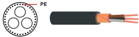
Symmetrical shielded cable with 3-ph. conductors and a concentric copper or aluminum PE conductor as shield (the shield must meet IEC 61439-1).
