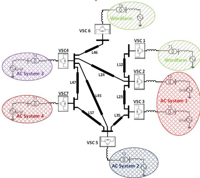
**Figure 9, A 7-terminal DC grid using Optimal Power Flow**
