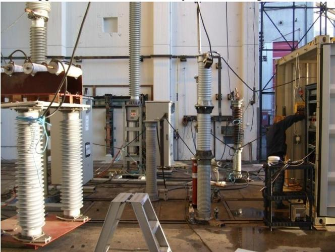
Figure 12, test setup for the mechanical HVDC breaker
