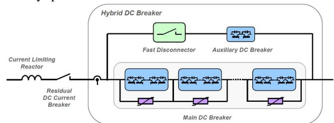
**Figure 10, The Hybrid HVDC Breaker concept**
