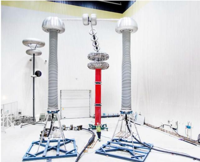
**Figure 7, Type testing of the 525 kV cable system**
