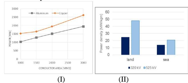
**Figure 8, (I) Transmitted power as a function of conductor area and metal for a cable pair, (II) Comparison of power density between a 320 kV extruded DC cable system and the 525 kV Al, 320 kV Cu).**
